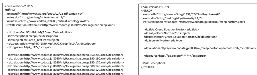
Fig. 2. Metadata description in RDF for (a) experimental data and (b) constitution equation. Data and equations are stored in XML files pointed by URI's
