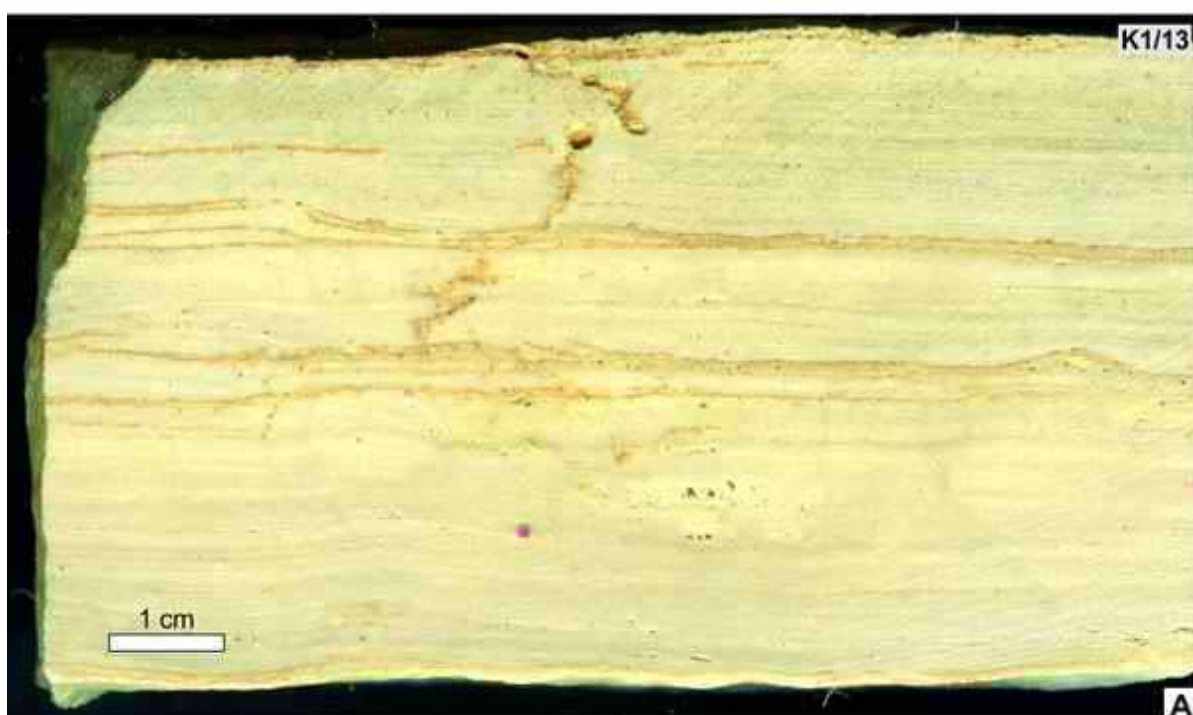
Outcrop K1. Unit K1/13, dolostone with “teepee” structure (A), (B) general view on the boundary between Member B (Sloisty Kamen (‘Laminary Stone’) Member), unit K1/13 and Member C (Podboi Member), unit K1/14, Rukovodyashchaya Glina (‘Marker shale’) of Noinsky (1899, 1924).
