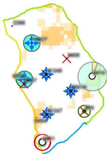
Figure 5. One of blocks of prediction map for site 1. Blue crosses mean injection wells, any color dots mean production wells, red and black crosses mean well was disabled. Brown color shows value of prediction - the darker the higher
