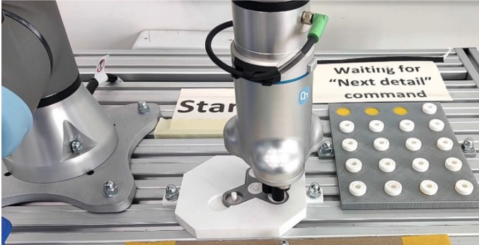
Fig. 4. The process of assembling the fidget spinner with the UR3e robot.
