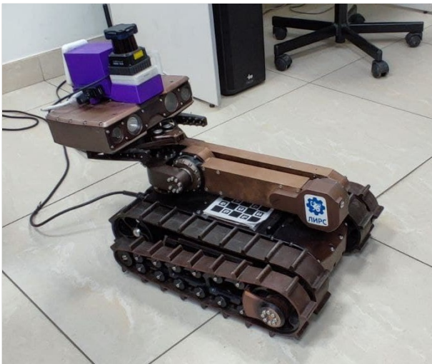
Fig. 1: Crawler Robot Servosila Engineer
