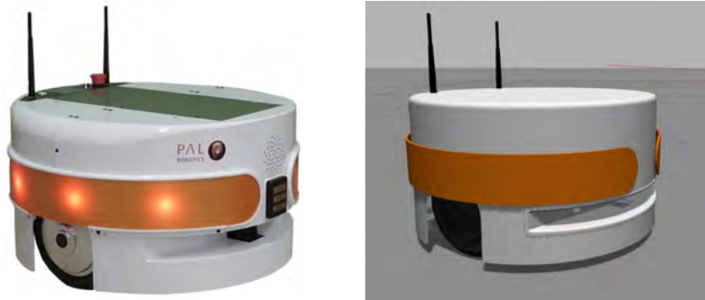
Fig. 3: The TIAGo Base mobile robot (left) and its model in the Gazebo simulator (right).
