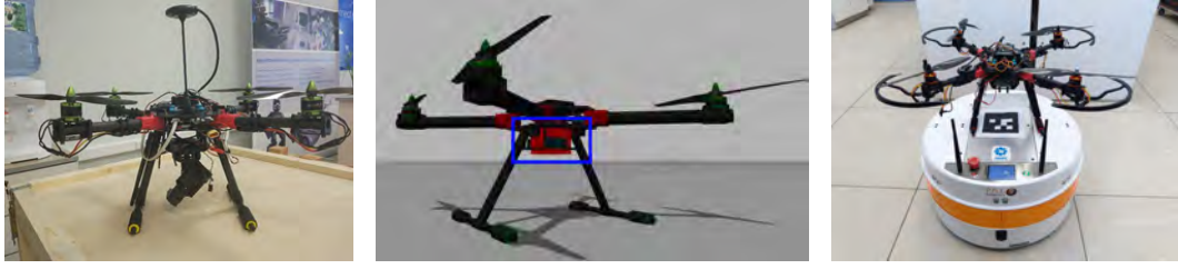
Fig. 4: The PX4-LIRS UAV (left) and its model in the Gazebo simulator with the RFID reader (middle). The RFID reader is highlighted with the blue rectangle. The TIAGo Base UGV with the ArUco tag 16h3 ID-198 on its top and the PX4-LIRS UAV (right).
