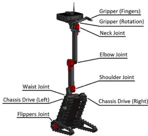
Fig. 1. Servosila Engineer servo drive scheme.
