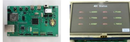
(a) IoT module main board (b) IoT module with LCD
