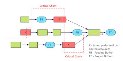
Fig. 5. Critical Chain in this case consists of tasks performed by limited resources.
