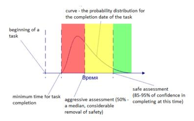
Fig. 1. Time of the completion of a task as distribution of probability.
